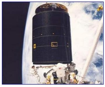
Once in orbit, Endeavour's crew got right to work setting up for the rendezvous with the Intelsat VI satellite – which was stranded and unusable in Low Earth Orbit following its launch on a Titan rocket in March 1990 when its launch system failed to place it in its correct, geostationary orbit.
