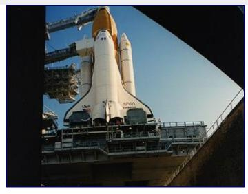
On August 18, 1994, Endeavour's launch countdown proceeded nominal. At T-31secs, the Ground Launch Sequencer handed off control of the countdown and Endeavour's systems to Endeavour's five General Purpose Computers (GPCs). At T-6.6secs, Endeavour's GPCs sent the commands to ignite the three SSMEs in reverse sequence (Engine 3, Engine 2, Engine 1).
