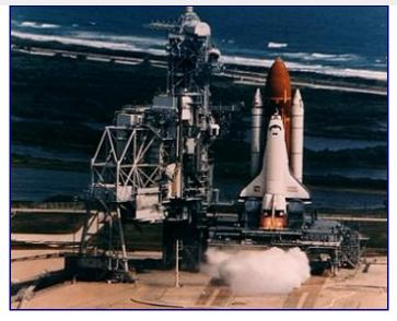
Five days later, on March 13, Endeavour and the STS-49 stack was rolled out of the VAB and out to Launch Complex 39B where pre-flight processing continued toward the planned Flight Readiness Firing (FRF) of her three Space Shuttle Main Engines (SSMEs).
